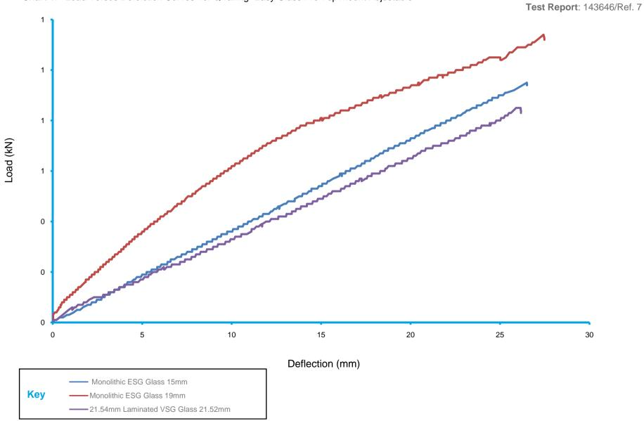
Chart 1: Load Versus Defelction Curves for Q-railing Easy Glass Pro Top Mount Adjustable
