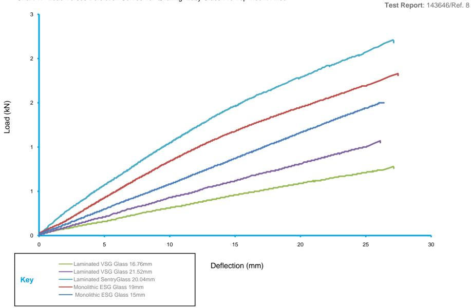
Chart 1: Load Versus Defelction Curves for Q-railing Easy Glass Pro Top Mount Fixed
